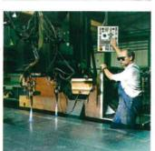
Manufacturing NC-Autogen flame-cutting systems max. cutting width:
