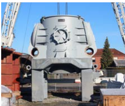
Service coal mill
